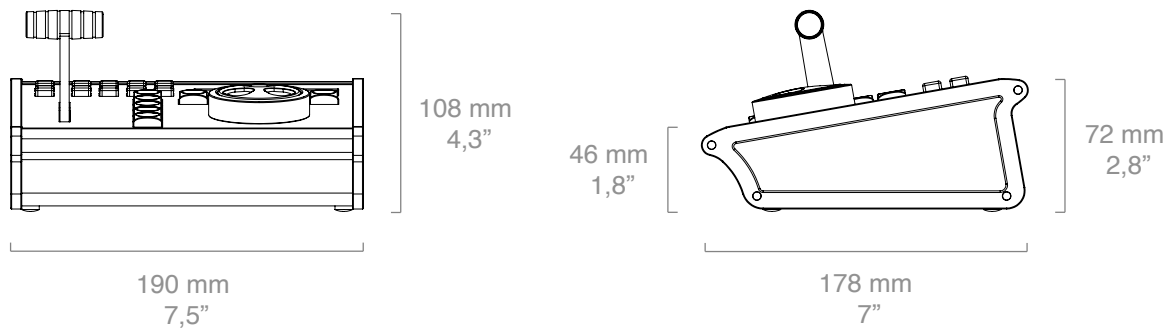
Figure 1: Technical drawing of Time Spin with key dimensions and layout details.
