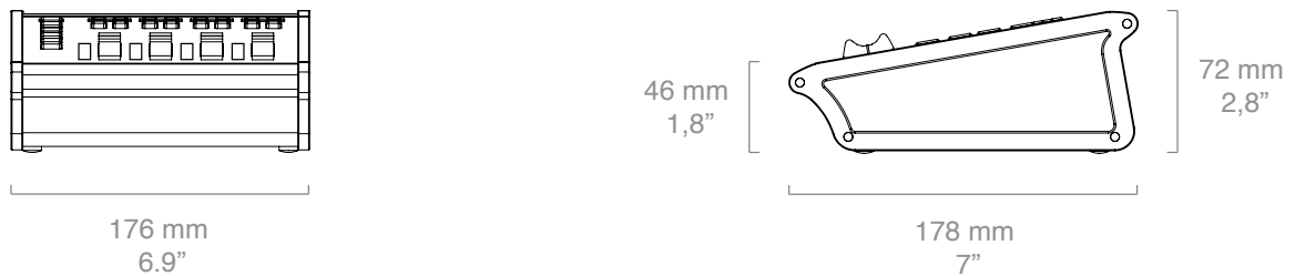
Figure 1: Technical drawing of Wave Board Mini with key dimensions and layout details.
